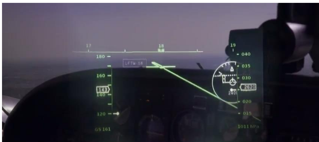
Figure 4: Example of decentred display of the destination runway, aiming point and extended centerline)
