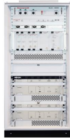
GBAS Technology: system overview graphics (left), ground subsystem Honeywell GBAS tower (right).
